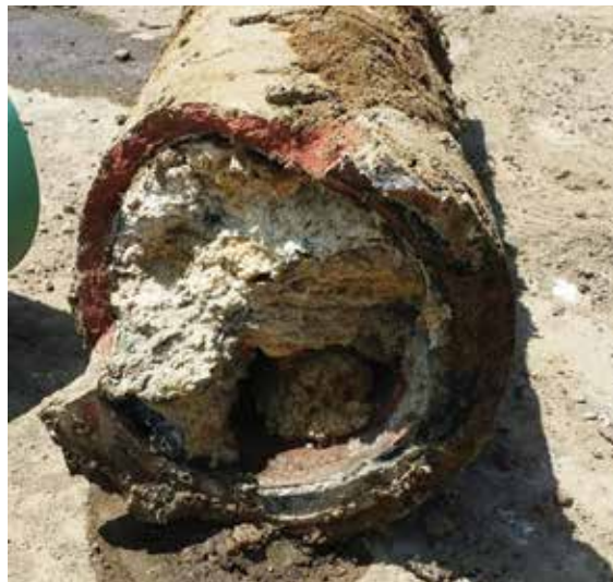
This sewer main was found to be completely clogged with grease in Madison, SD.
